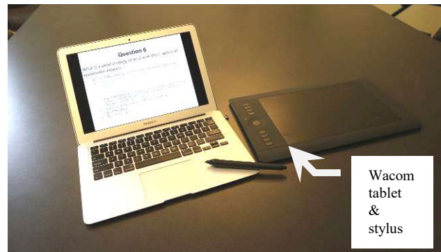
Figure 2 Wireless Wacom Intuos Pro tablet (right) for annotating PowerPoint slides on a Macintosh laptop (left).
